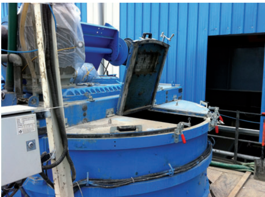
A 1cbm planetary mixer from Sicoma is producing the concrete in Hosur
