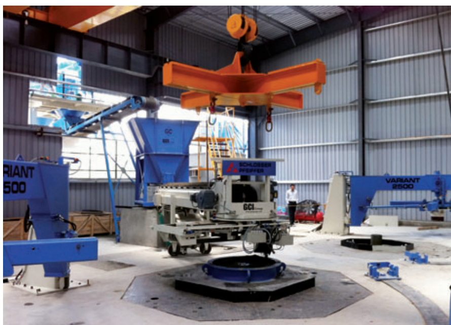
With the new Variant 2500 D production machine from Schlosser-Pfeiffer, the facility is the biggest pipe plant in South India
